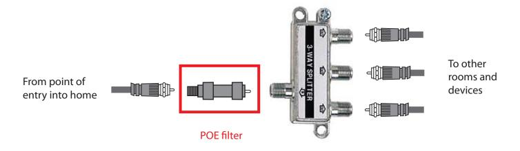
3. Check to make sure your MoCA network is still functioning properly. If it's not, the POE filter is likely installed in the wrong location. Be sure to install the filter as close as possible to the point where the cable signal enters your home (not after it splits into different rooms).
